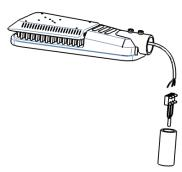
2. Please loosen the screw to fix the pole on the fixture and then insert the fixture into the pole. 用扳手松开路灯上的灯杆固定螺丝,将路灯插到电线杆子上;
