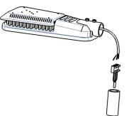
2. Please loosen the screw to fix the pole on the fixture and then insert the fixture into the pole. 用扳手松开路灯上的灯杆固定螺丝,将路灯插到电线杆子上;
